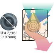
Large cross flow fan – A new and improved fan design delivers higher performance with lower energy consumption and whisper-quiet operation as low as 19 dB(A). Greater airflow up to 453 CFM delivers greater temperature stability throughout the conditioned space.
